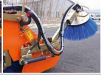
Hydraulic side brush w/hydraulic lifting and lowering
